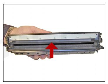
12. Vacuum the doctor blade and foam feed roller clean. We do not recommend that the doctor blade be removed and the developer roller felt seals will be disturbed. Once a new blade is available, great care will have to be taken not to tear the seals, causing a leak. The doctor blade can be easily cleaned by blowing the excess toner off, and wiping down with a lint free cloth. Be very careful not to leave any lint behind!
