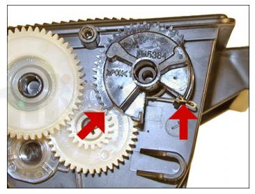
18. Set the reset gear and spring as shown. The straight tail of the spring fits into a notch at the base of the gear shaft.
