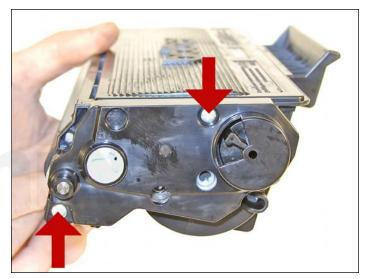
4. On the gear side, remove the two screws and cover plate.
