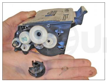
5. The black spring-loaded reset gear may fall off as the plate is removed. This gear resets the printer when the cartridge is installed. New starter cartridges do not have this reset gear. Until they are available, the starter cartridges cannot be remanufactured.
