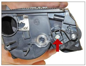
20. Install the drum axle plate on the non gear side and screw.
