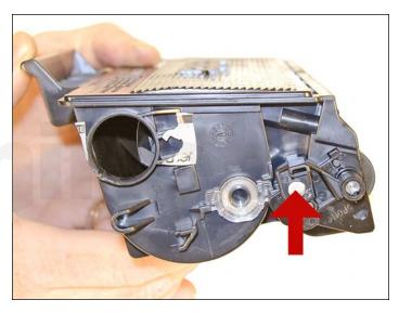
2. On the non-gear side of the developer roller, remove the screw.
