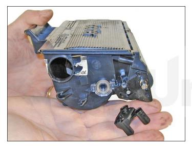
3. Remove the drum axle plate.
