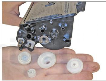
8. Remove all the remaining gears.
