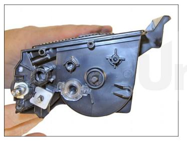
16. Clean the gears, making sure that they have no toner on them. This is a good time to also check the gear shafts to make sure there is enough grease. If the shafts appear dry, or the grease is contaminated with toner, clean the shaft and inside of the gear. Replace the grease with white lithium grease.
