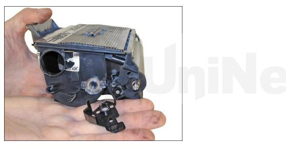
9. Remove the non-gear side end cap by gently prying it off.
