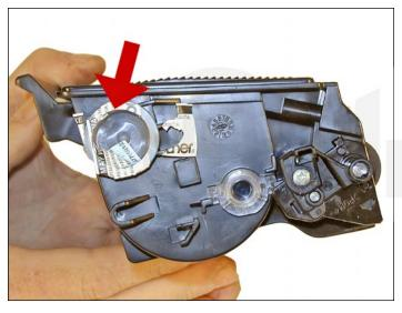
1. Vacuum the exterior of the cartridge. Remove the fill plug from the toner cartridge. Dump the remaining toner and vacuum/blow out the cartridge. Make sure that the gear area is clean. Leaving any toner in the teeth of the gears may cause a tooth to be damaged and cause a clicking noise. We have found it best to use compressed air to clean them out, but to also keep one hand over the gears to protect them.
