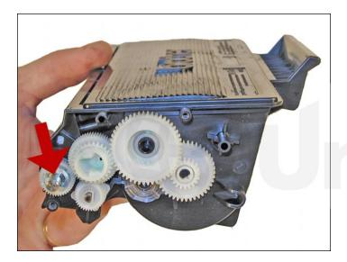
7. Remove the E-Ring, and small gear.
