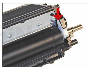
14. Clean the developer roller with a lint free cloth. Do not use any chemicals other than a dedicated cleaner for the Brother rollers to clean the roller. A dry clean cloth will work fine. Re-install the developer roller long shaft side to the gear side, and white lock pointing up. Turn the lock towards the doctor blade until it locks in place.
