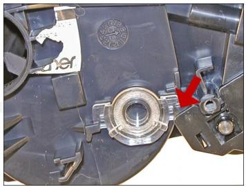
15. Install the small outside end plate on the non-gear side.
