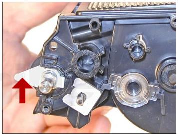
10. On the gear side of the developer roller, press in on the locking tab and rotate the developer roller lock up.
