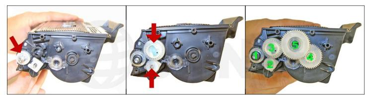
17. Install the developer roller gear, c-ring, black axle and the rest of the gears.
