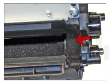
13. Inspect the magnetic roller felts. If they are compressed (shiny), roughen them up with a small screwdriver.
