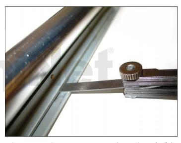
6. It is best not to take the doctor blade assembly apart, but if you do, use a gapping gauge to measure the gap by each of the five screws before removing any of them. Set the gap back to the proper distance when re-assembling the blade assembly.
