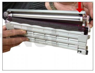
2. Lift up on the doctor blade side and remove the developer roller assembly.
