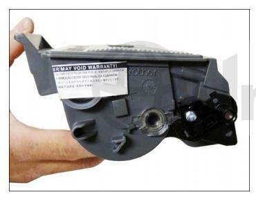
1. Vacuum the exterior of the cartridge. Remove the fill plug from the toner cartridge. Dump the remaining toner and vacuum/blow out the cartridge. Even though the gears are covered on these cartridges, we have found it best to keep one hand over the gear side to protect them.
