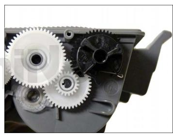
15. Depending on the cartridge you have, set the reset gears as shown:
