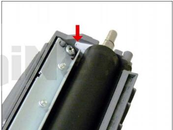
12. Re-install the developer roller long shaft side to the gear side, and white lock pointing up.
