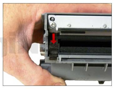
11. Inspect the magnetic roller felts. If they are compressed (shiny), roughen them out using a small screwdriver. Clean the developer roller with a lint free cloth. Do not use any chemicals other than a dedicated cleaner for Brother rollers to clean the roller. A dry clean cloth will work fine.
