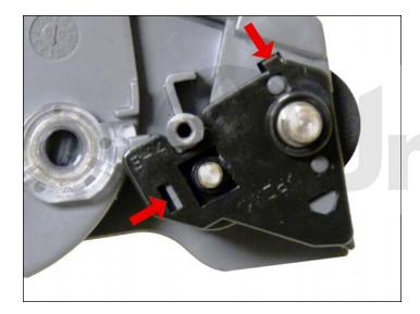
3. Remove the drum axle plate by pressing on the two tabs as indicated. Pry the plate off.
