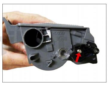
2 On the non-gear side of the developer roller, remove the screw and outer axle cover.
