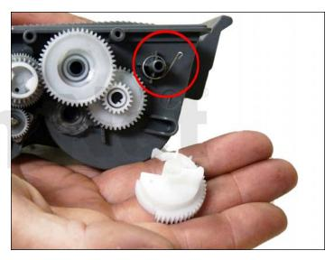
5. The reset gear is spring-loaded and must be positioned correctly for the printer to accept a new cartridge.
