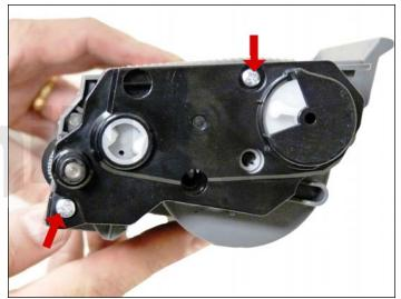
4. On the gear side, remove the two screws and cover plate.
