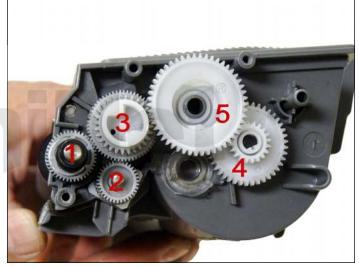
14. Install the developer roller gear, E-ring, black axle spacer, and the rest of the gears in the order shown.
