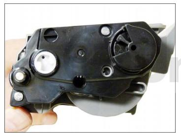
16. Install the gear cover plate and two screws:
