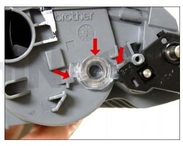
13. Install the non-gear side axle plate. Make sure the clear plastic plug for the optical sensor is locked in the proper position. Clean the gears making sure that they have no toner on them. This is a good time to also check the gear shafts to make sure there is enough grease. If the shafts appear dry, or the grease is contaminated with toner, clean the shaft and inside of the gear. Replace the grease with white lithium grease.
