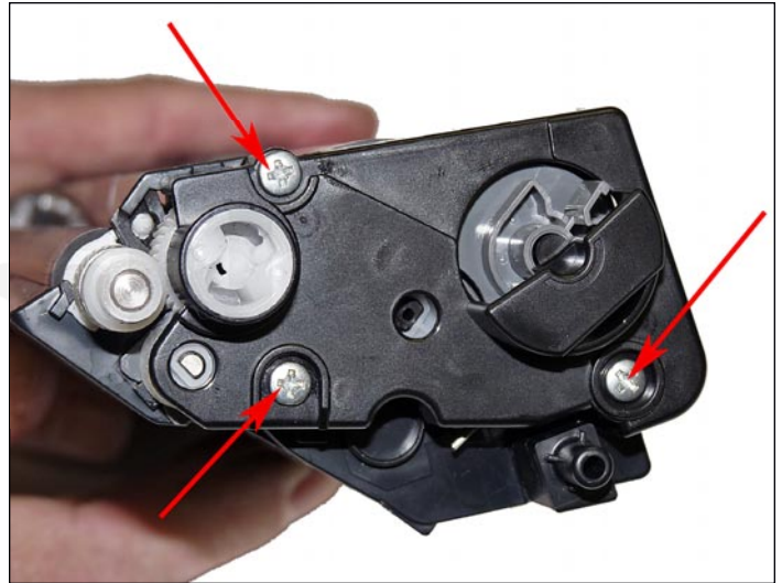
26. Install the gear cover plate, and three screws.
