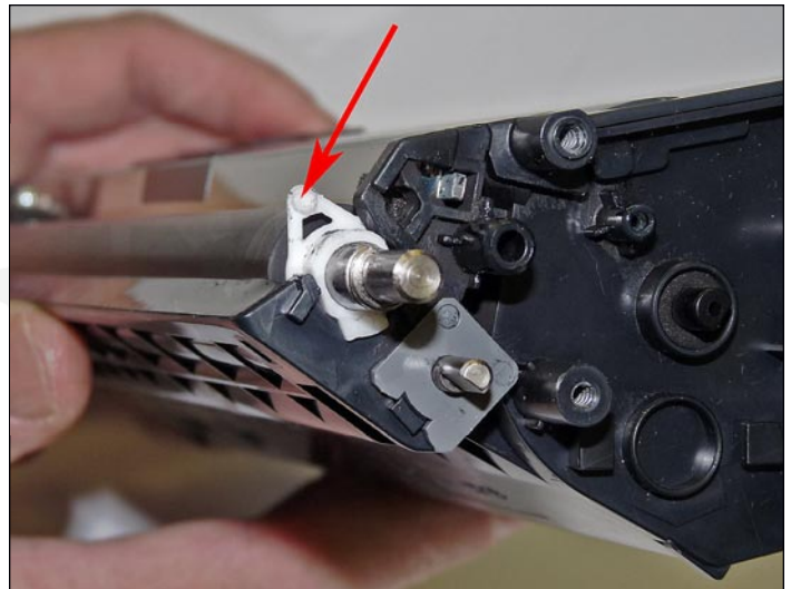
10. Move the white plastic locking tab on the right side of the developer roller to the up position.
