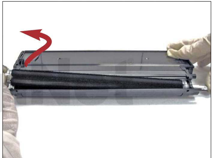
15. Remove the magnetic roller and clean using compressed air to blow off all the remaining developer.
