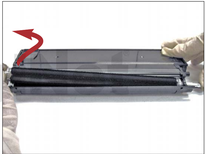
13. The fastest way to remove the support bearing on the opposite side is to first lift the magnetic roller. Pull it out about 5mm, then stop and position the magnetic roller back in the cartridge
