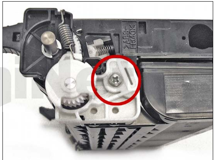
3. Remove the screw from the white end cap.
