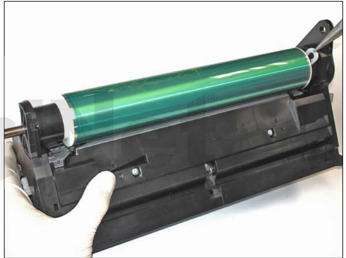
44. Install the new or recycled lubricated drum, the white U-shaped clip, the axle with new conductive grease lubricating the dedicated contacts, and the plastic black drum gear cover. Be mindful of the inside drum contact. Check it with a hook tool.
