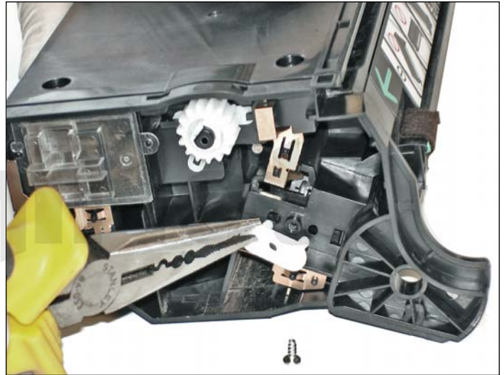
18. Remove the white plastic corona supports on both sides.
