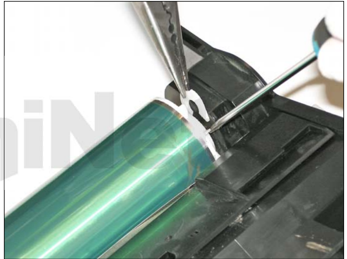
10. Remove the plastic white clip from the drum shaft.
