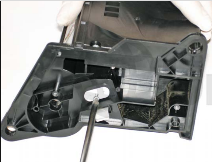
17. Unscrew both Phillips screws from the white plastic corona support on each side of the cartridge.
