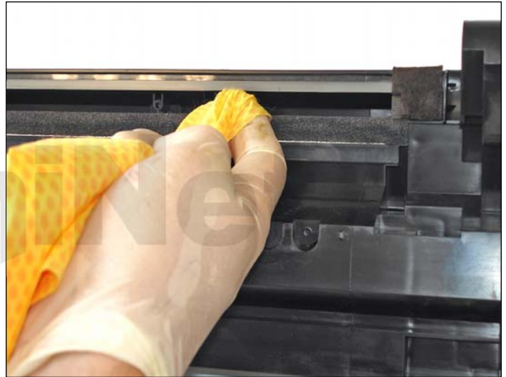
36. Clean the recovery blade with a cotton tip swab or magnetic toner cloth with alcohol isopropyl mixed with distillate water. Be careful not to damage or bend the blade since it would cause spotting.
