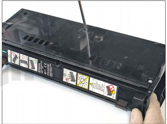
30. Remove the six larger top chamber cover screws.
