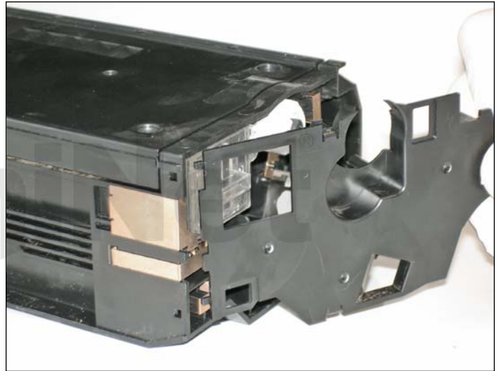
16. Remove the whole black lateral end cover lifting it as shown. Otherwise, the tabs can be damaged.
