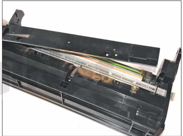
20. Release the black long end cap cover carefully.
