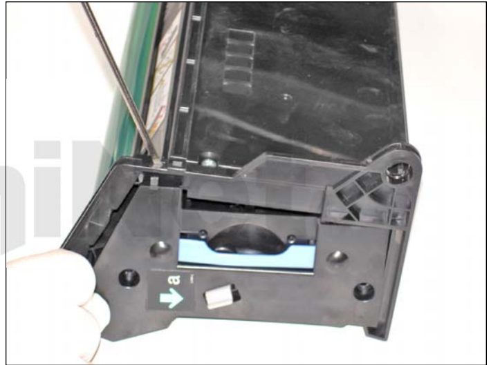
8. Using a small flathead screwdriver, press in on the upper black end locking tab to release the end cap.
