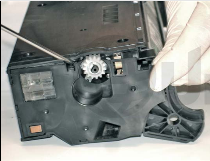
15. Using a hook tool, unlock the gear end plate tab on the opposite end of the drum unit.
