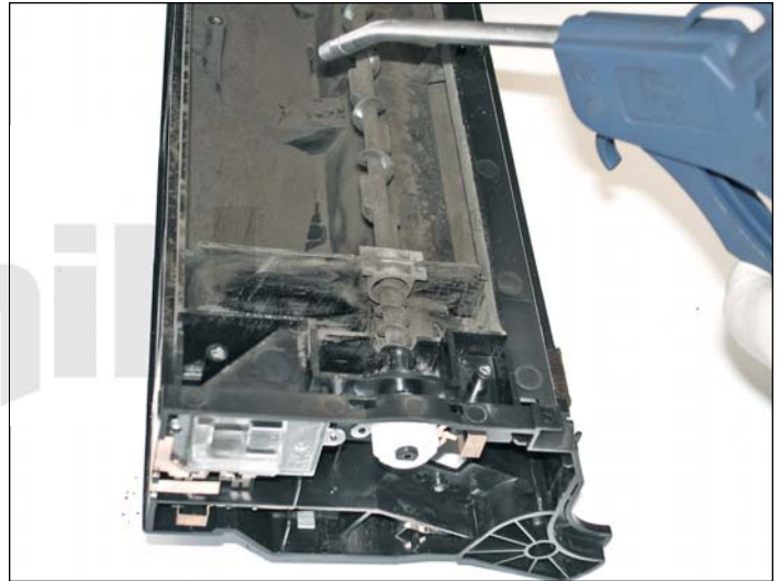
32. Clean the waste hopper with compressed air.
