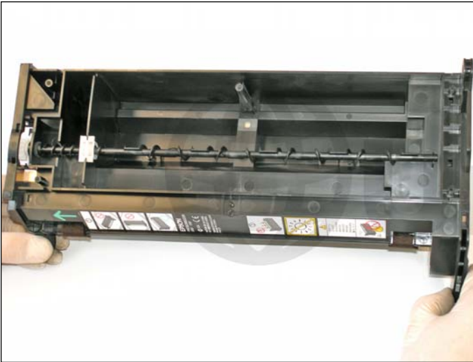
33. General view once cleaned. Clean as best as possible the plastic yield sensor window placed in the waste toner section to avoid a "full waste toner" message on printer's display.
