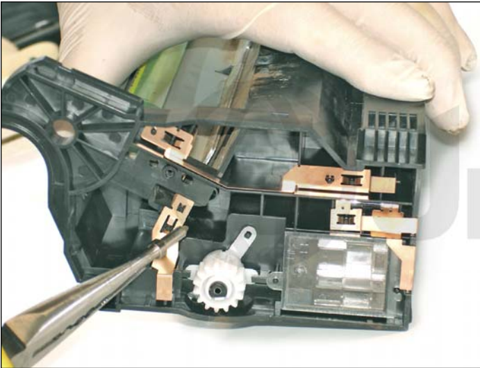
27. Release the second wiper blade blocking pin with the same procedure.
