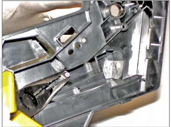
24. Remove the lateral wiper blade blocking pin from one end of the cartridge using needle flathead pliers.
