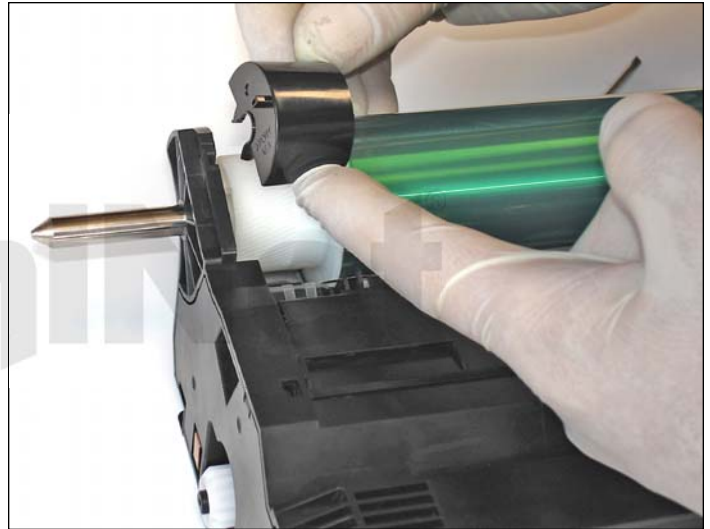
12. On the opposite end, remove the plastic black drum gear cover shown.
