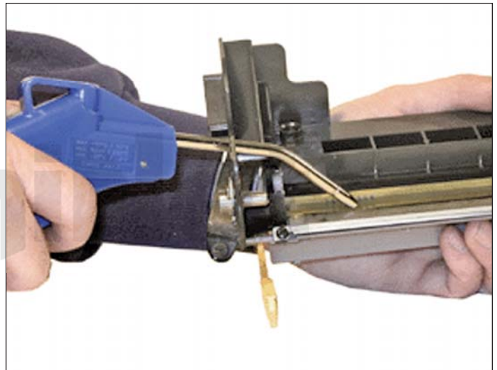
5. If you are not replacing the wiper blade, tap the waste chamber upside down and vacuum/blow off any remaining toner.
