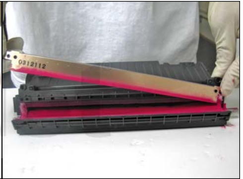
15. Remove the two doctor blade screws, and doctor blade. Clean the doctor blade with a lint-free cloth, and apply a small amount of pressure. Do NOT use any chemicals.
