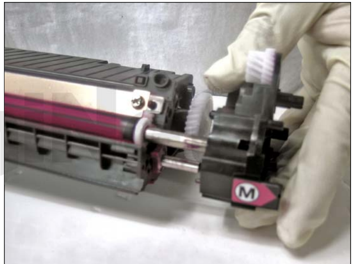
12. Remove the two screws on the roller support assembly, then slide it out.
