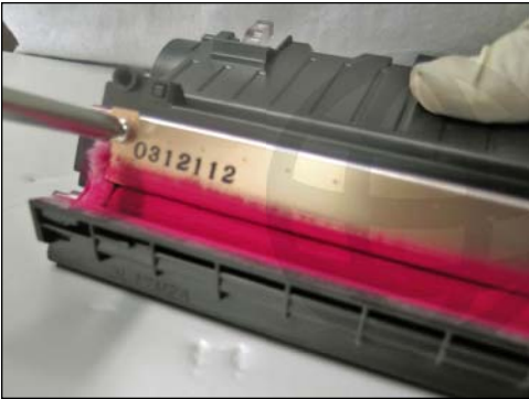
15. Remove the two doctor blade screws, and doctor blade. Clean the doctor blade with a lint-free cloth, and apply a small amount of pressure. Do NOT use any chemicals.
