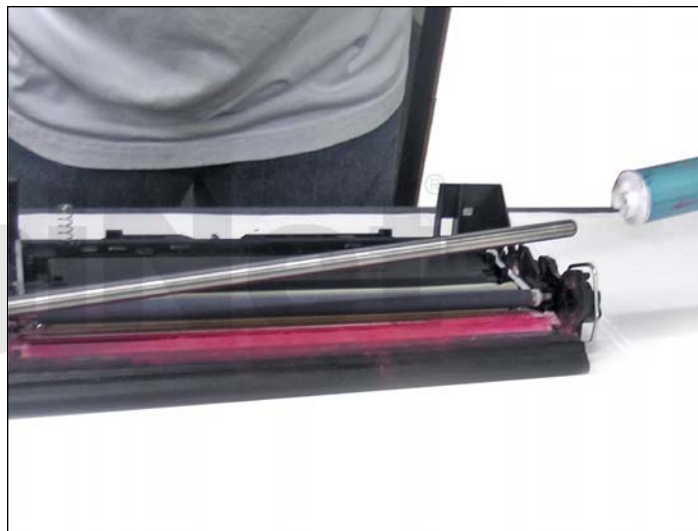
28. Slide out the drum as shown.
