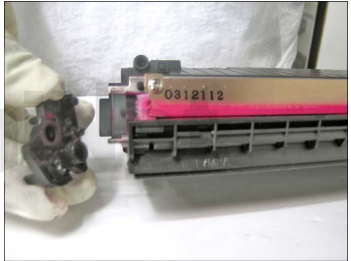
14. Remove the two roller support plate screws, and roller support plate on the contact (gearless) side.
