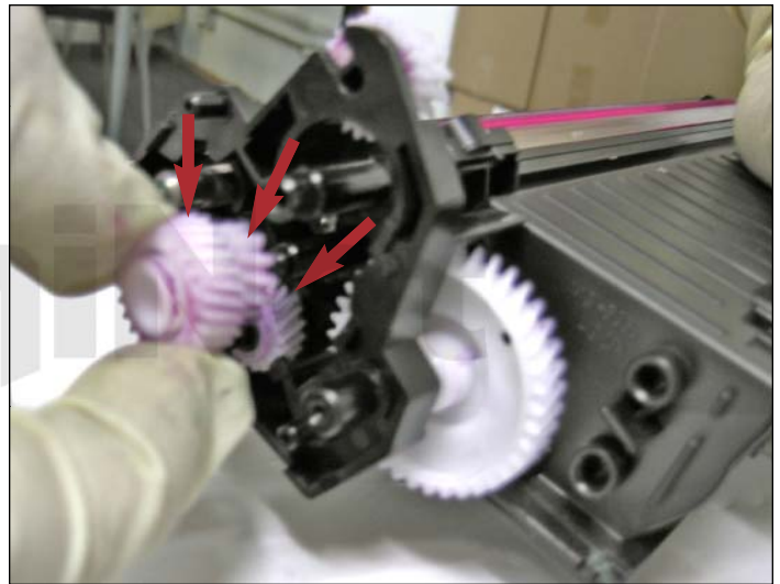
11. Remove the three small inner gears shown.
