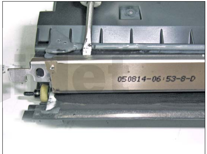
23. Using a small flathead screwdriver, pry the the doctor blade loose from the OEM adhesive. Pry loose from one side only!
