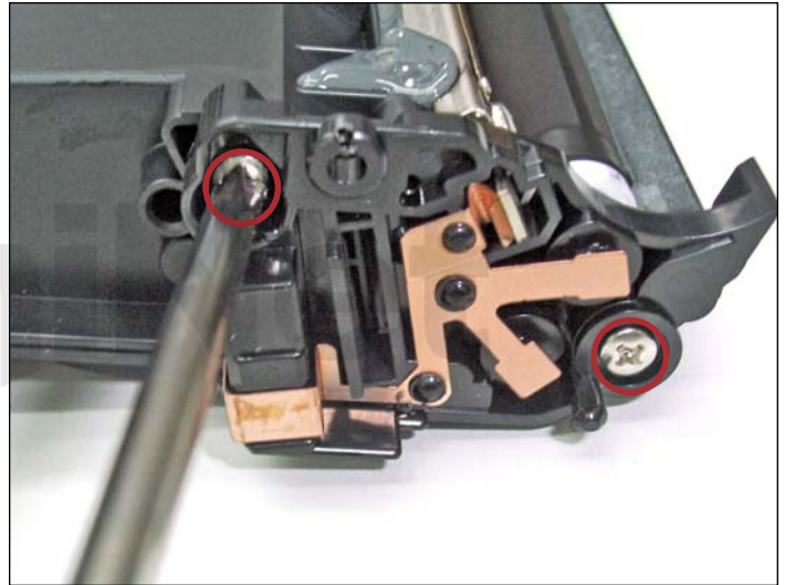
19. Remove the two screws from the developer roller gearless support plate on the contact side of the cartridge.
