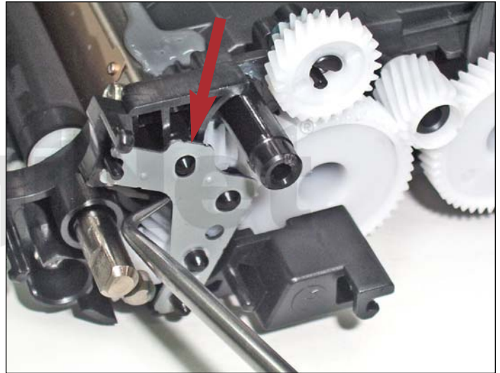
15. Using a hook tool, slide out the gear retaining plate.
