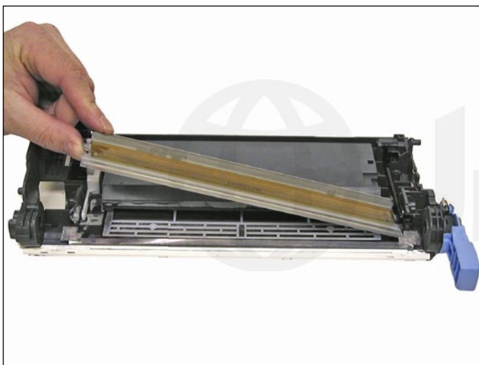
14. Remove the wiper blade.
