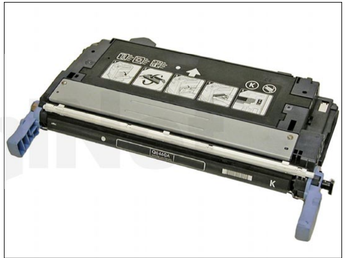
43. Place the supply chamber onto the waste chamber.
