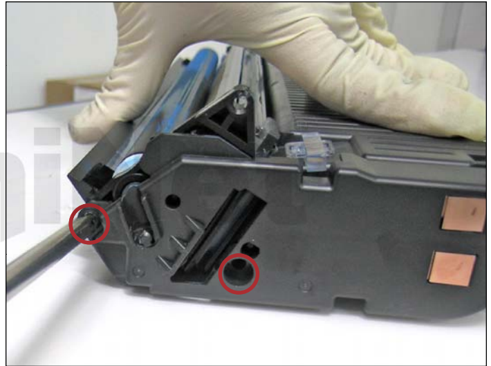
15. Remove the two screws on the contact side (gearless).
