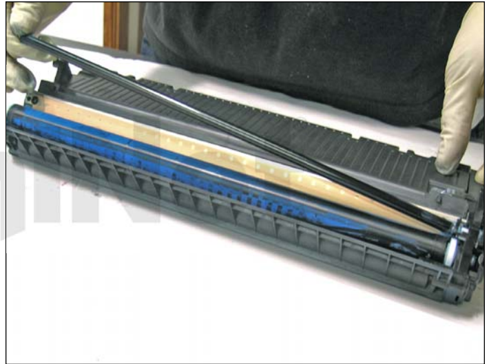
19. With the gear side support plate removed, you can now remove the toner charging roller.
