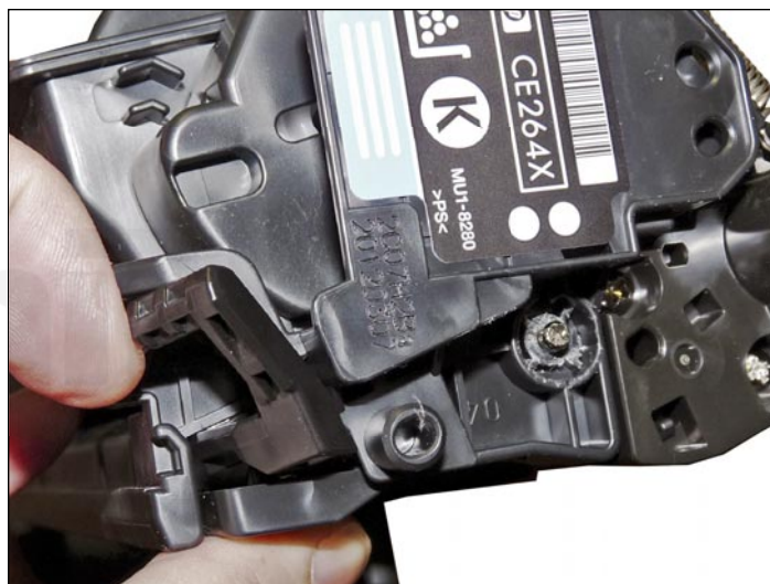
6. On the opposite side, lift up on the black lever.
