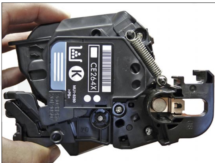
47. Install the spring.
