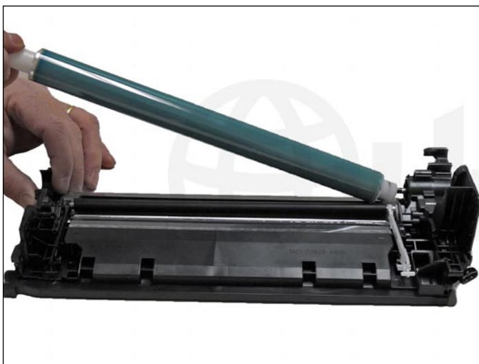
8. Remove the drum.
