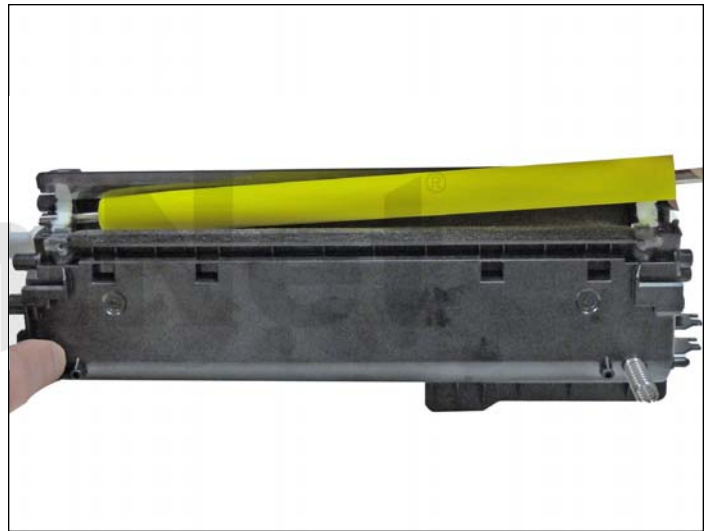
30. Remove the feed roller.
