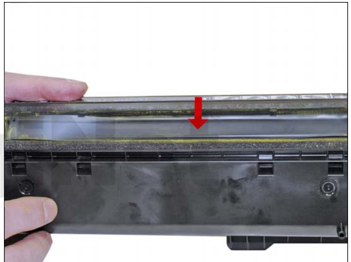
32. When a seal is available, install the seal onto the seal rails. Pull the release tape off one-inch at a time and press the seal in place as you go.
