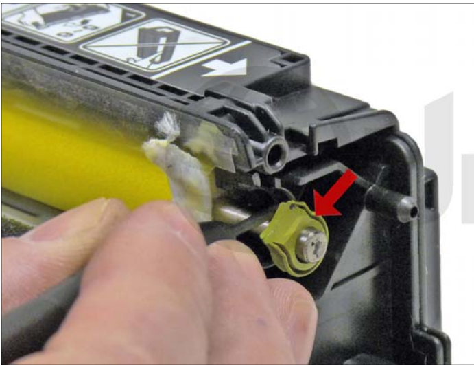
29. Pry out the rubber feed roller bushing from the right side.
