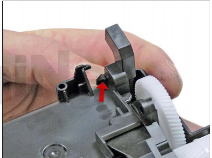
19. Press in on the tab and remove the end cap.
