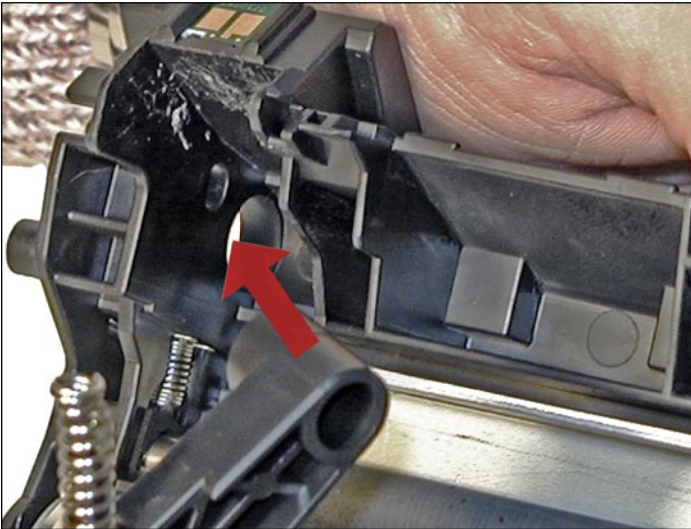
25. Place the drum/waste hopper into the toner hopper.
