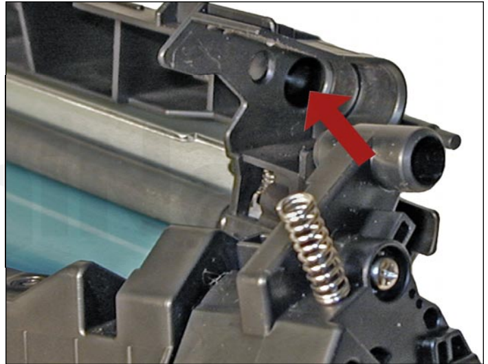
25. Place the drum/waste hopper into the toner hopper.
