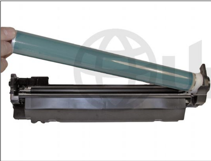
7. Remove the photoconductive drum.
