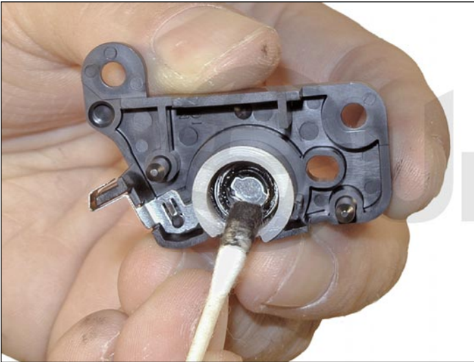
22. Clean the mag roller contact plate on the contact end cap.
