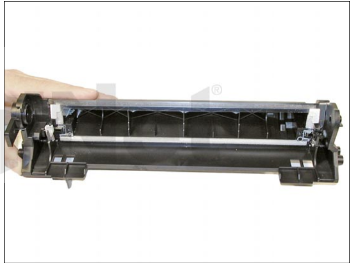
10. Clean out any remaining waste toner. Make sure the foam seals under the wiper blade are clean and not damaged.
