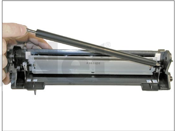
8. Remove the primary charge roller (PCR), by prying it out of the clips on either end. Clean the PCR with your preferred cleaner and place aside.
