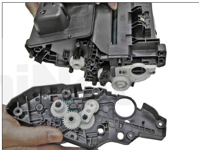
6. Remove the right and left side end caps from the cartridge. Note that the gears do not come off the gear (right) end cap.
