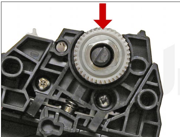
34. Install the magnetic roller sleeve drive gear.
