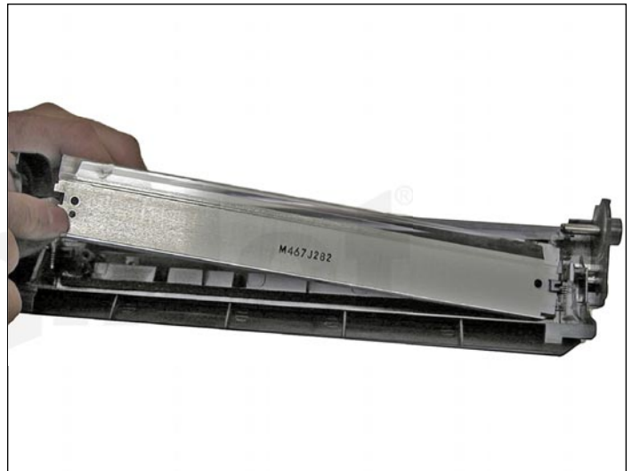
12. Remove the wiper blade from the cartridge and clean out the waste toner.
