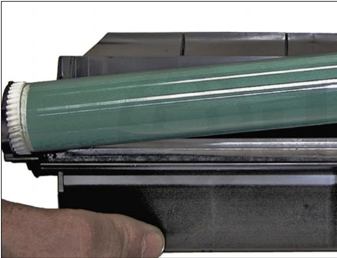
17. Install the drum small gear side first onto the drum axle pin.
