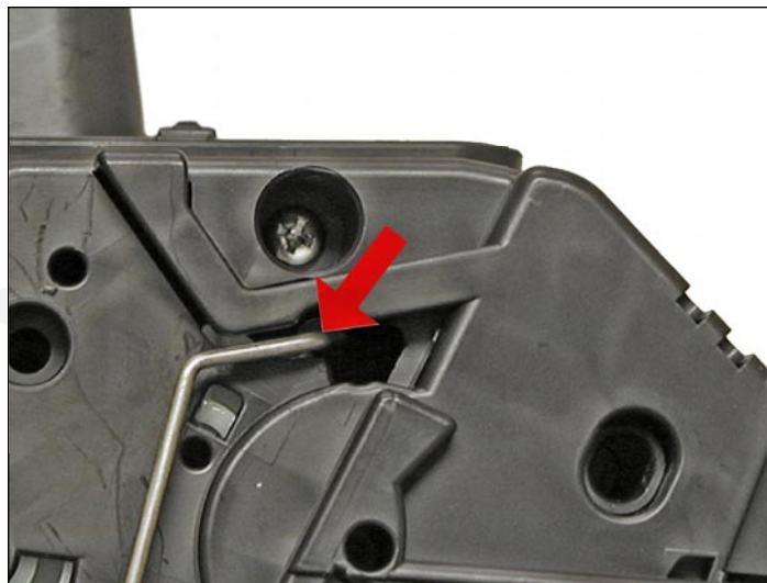
41. Install the metal bars from the drum cover on both sides of the cartridge.
