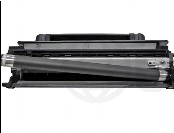
23. Remove the magnetic roller sleeve assembly.
