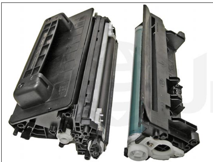
7. Separate the toner hopper and waste chamber.
