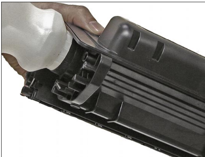
36. Fill with appropriate amount of new replacement toner for use in P4015. Install the fill plug.
