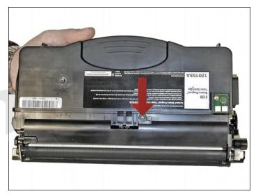
23. Install the developer roller cover and screw.
