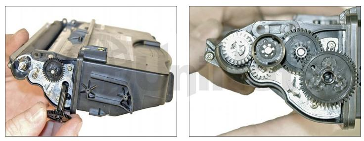
19. Install the gears. The large gear with the long shaft fits onto the toner agitator bar inside the hopper. Spin it a few times and listen to make sure it is engaged properly. On the large drive gear, make sure the flat washer is in place, and install a new star lock washer. Make sure the lock washer is pressed down fully against the base of the gear.
