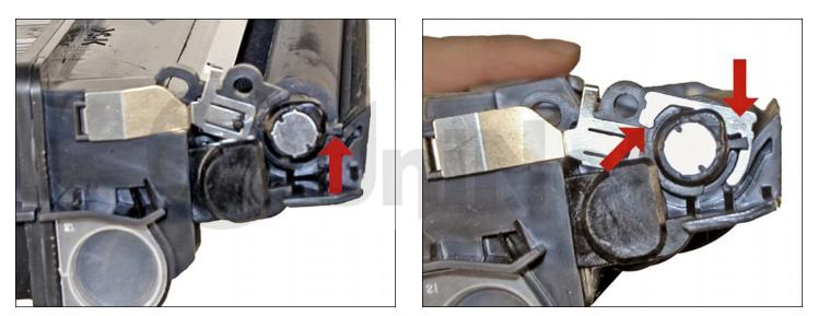
16. Reinstall the developer roller. Spin the plastic bushing so it is locked in place.
