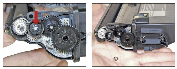
7. On the large black drive gear, there is a locking star washer pressed onto the shaft. With a small pair of wire cutters, cut the old washer off, and remove. You can try to bend up the different legs of the washer, but that is very time consuming, and most likely at least one leg will break anyway and the washer will still have to be replaced.
