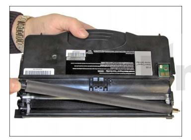
14. Lift the developer roller out of the cartridge.
