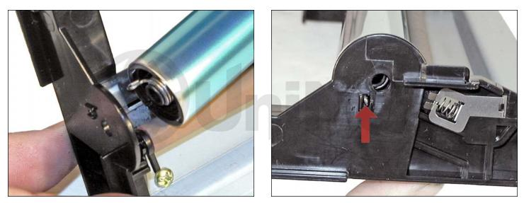
35. Coat the drum with your preferred lubricant, install the drum.
