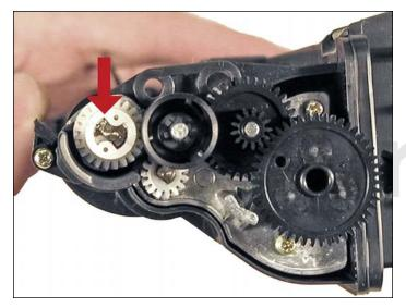
20. Lastly on the developer roller drive gear, spin the gear by the two small holes while holding the developer roller in place. This will lock the gear on to the shaft.
