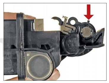
13. Turn the developer roller bushing so the plastic tab is facing up.
