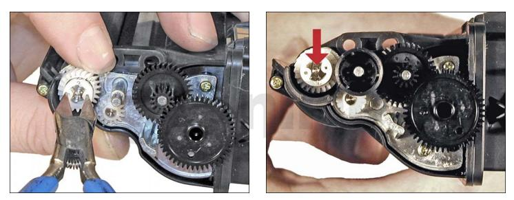
9. On the white developer roller gear, take the tips of your small wire cutters, and place them into the two small holes.
