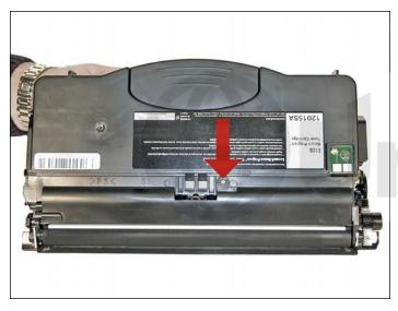
3. Remove the center screw on the developer roller cover.
