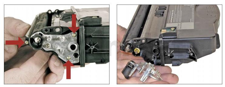
11. Remove the three screws and gear alignment plate.
