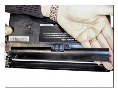
4. Lift up the developer roller cover from the center, and remove.
