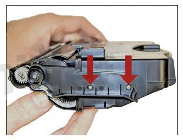
2. On the left side, remove the two small screws and the gear cover.
