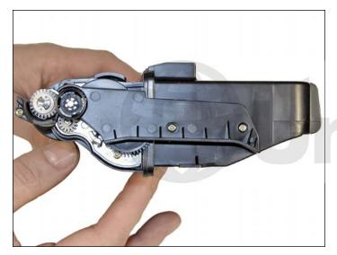
24. Install the gear cover and two screws.
