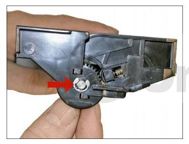
**DRUM CARTRIDGE** 28. On the gear side of the drum unit, remove the E-ring from the drum axle shaft.
