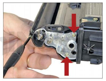
18. Install the gear axle plate and three screws.
