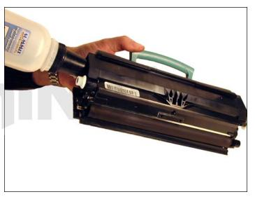
14. Fill the cartridge with the proper amount of toner and install fill plug.
