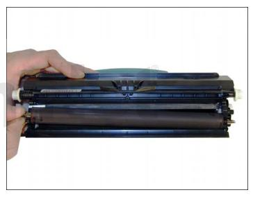
9. Wipe the developer roller with a clean lint free cloth, and re-install the developer roller. At this point we do not recommend that any chemicals be used to clean this roller. Install the keyed end of the roller to the gear side.
