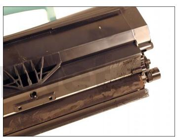
Left image shows the cartridge with the new felt style cover. Right image shows a sample of the leakage found on just about every cartridge tested so far. None of the leakage showed on prints past the first or second pages, but it did show.
