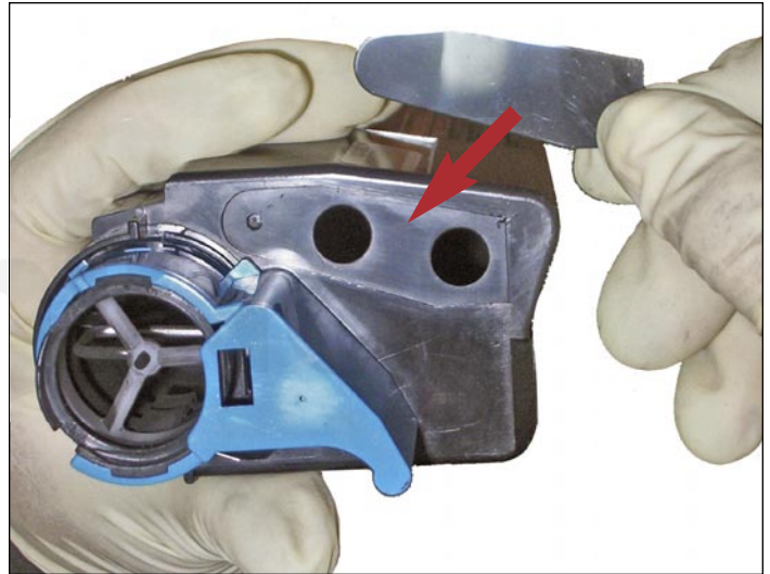
30. After cleaning use alcohol to clean both the cartridge and the tab openings, then reinsert the adhesive tab.
