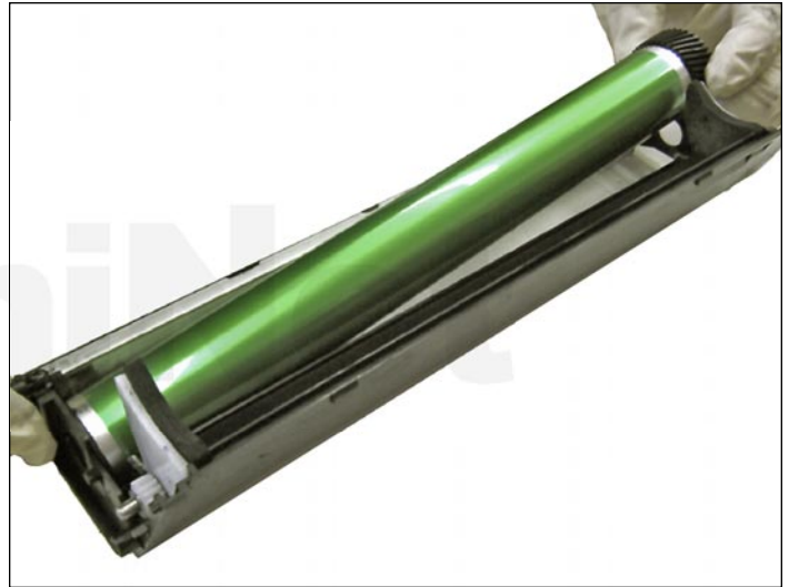
18. Carefully remove the drum as shown (gear side first).
