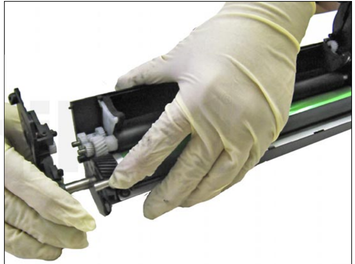
12. Slide the loosened small end cap out.
