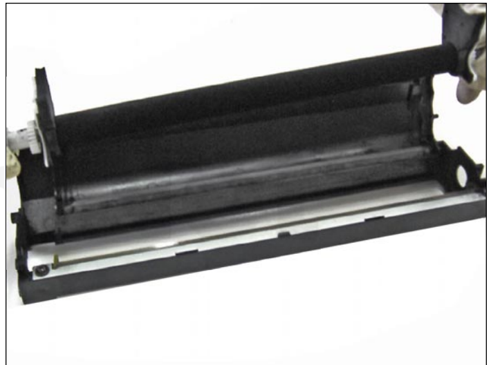
20. Remove the supply roller and its components shown.
