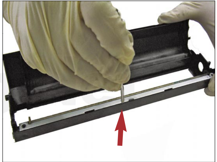
22. Gently pry the wiper blade up from the locking clip, using a small flat head screwdriver.
