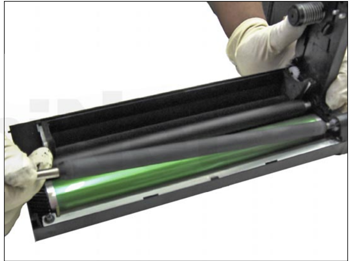
14. Remove the primary charge roller (PCR).
