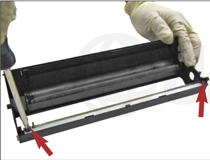
21. Remove the two wiper blade screws shown.
