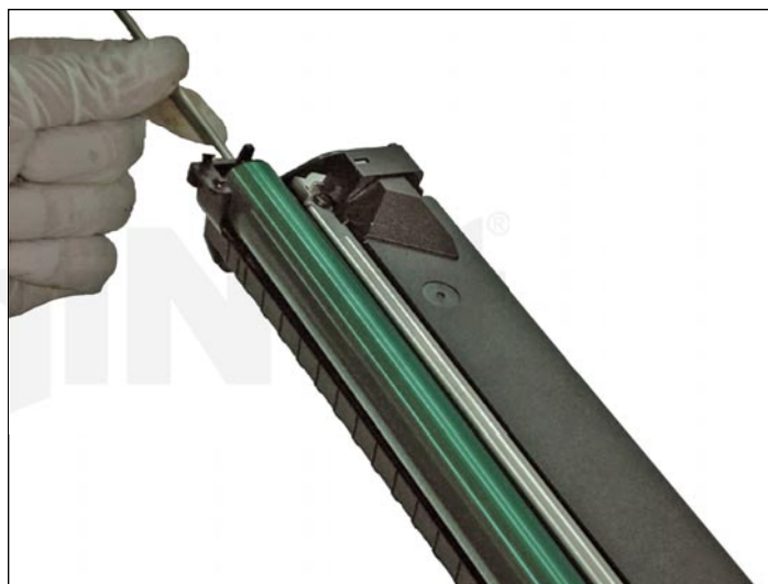
14. Clean and then install the OPC in position. Slide the OPC axle in with the keyed end first from the hub side (left) toward the gear side (right). Turn the axle slowly while pushing. Set unit aside.
