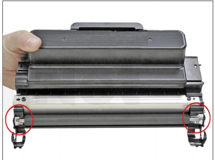
32. Clean the developer roller with a dedicated developer roller cleaner, and replace into the hopper. Place the long shaft side to the gear side of the cartridge. It should snap in place if installed correctly.
