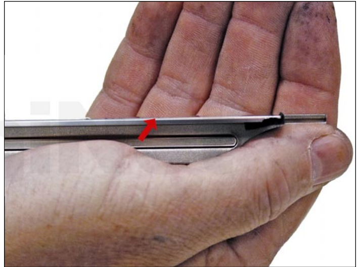
28. Clean the doctor blade edge so there is no evidence of build up along the edge. If any buildup exists, the cartridge will streak. No chemicals should be used. We have found using a clean, wooden ice cream-type stick works great for scraping the blade clean without damaging it.
