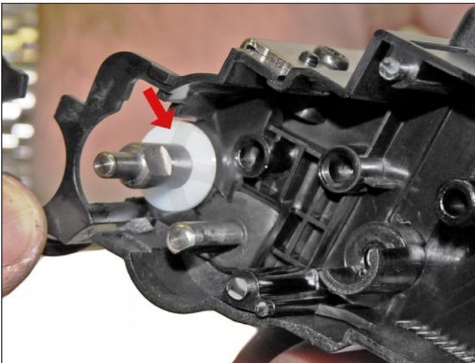
24. Remove the developer roller bushings from both sides.
