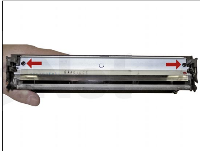
19. Install the new wiper blade and two screws.
