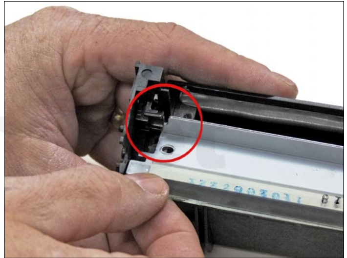
11. Remove the two screws from the wiper blade, and remove the blade.
