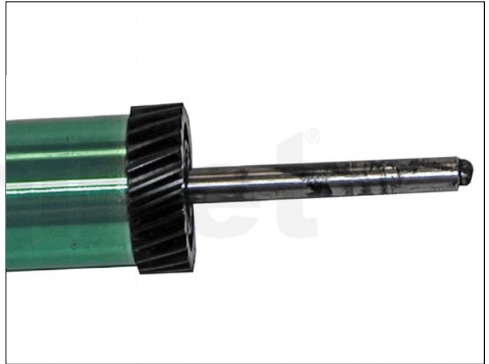
13. The gear side of the drum axle shaft has conductive grease on it. Regardless of if you are replacing the drum or not, clean the old grease off, and replace with new.
