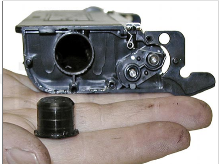
15. Carefully pry out the fill plug on the toner hopper, and dump out any remaining toner. The fill plug can be difficult to remove. Take a small common screwdriver and work it around the edge lifting slightly until it comes loose.
