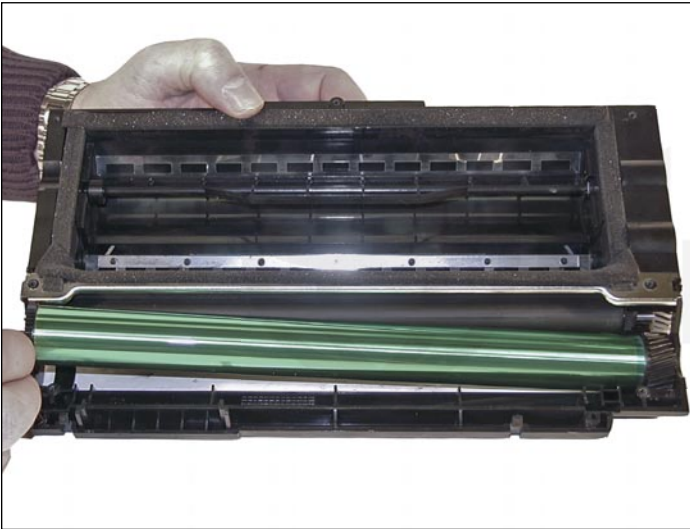
19. Install the new drum in place.
