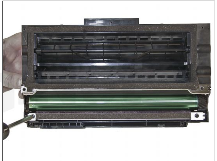
20. Install the PCR cleaner assembly.
