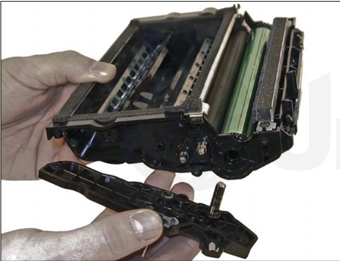
21. Clean the conductive grease off the left side (non gear) end cap and replace with fresh grease. Replace the end cap and four screws.
