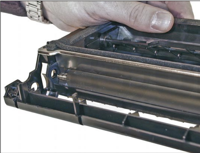
15. Replace the developer roller, and flat washers.
