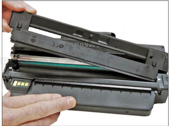
7. Separate the two halves slightly, and lift off the middle top cover.
