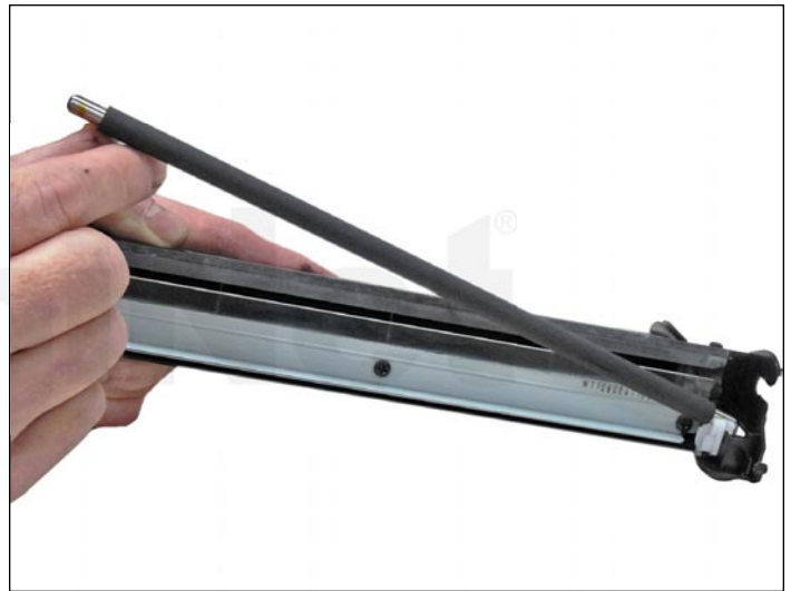
10. Remove the primary charge roller (PCR) from the assembly. Clean the PCR with your normal PCR cleaner.
