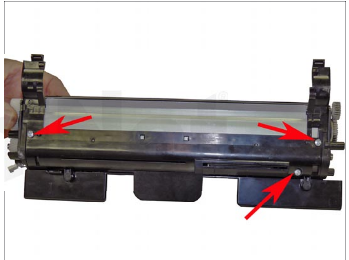
31. Install the bottom cover and three screws.
