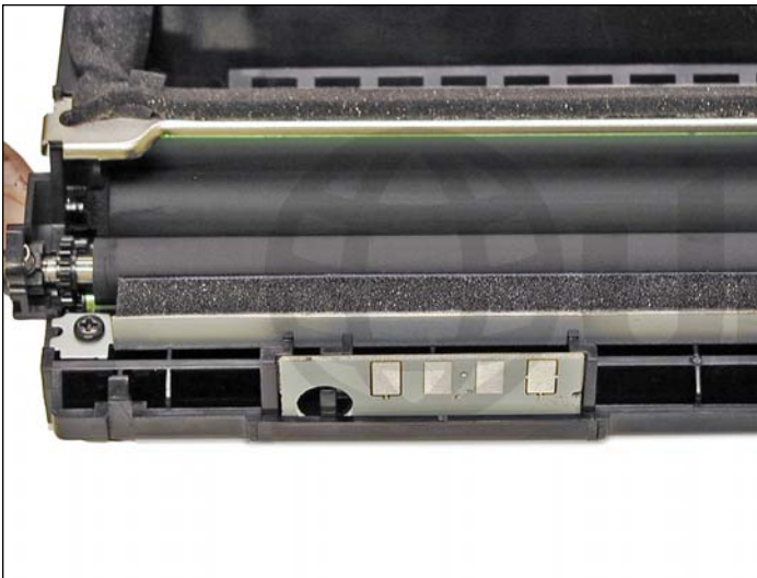
20. Replace the chip inside the top cover.
