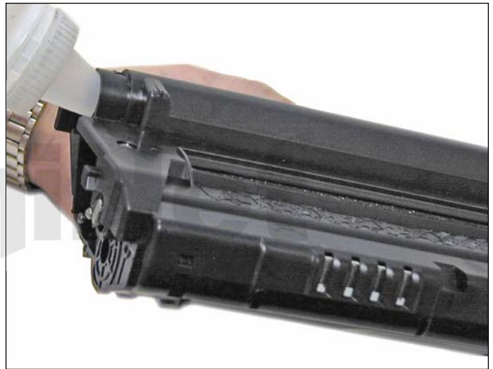
23. Fill the hopper with toner for SCX-4300.
