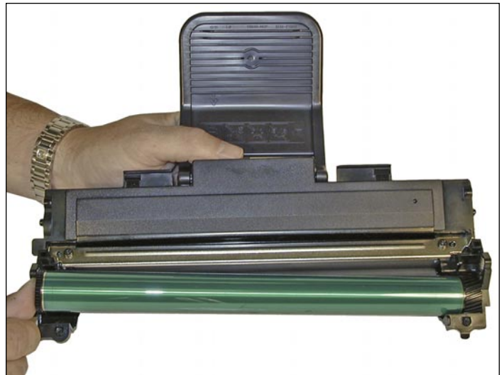
20. Install the drum in place.
