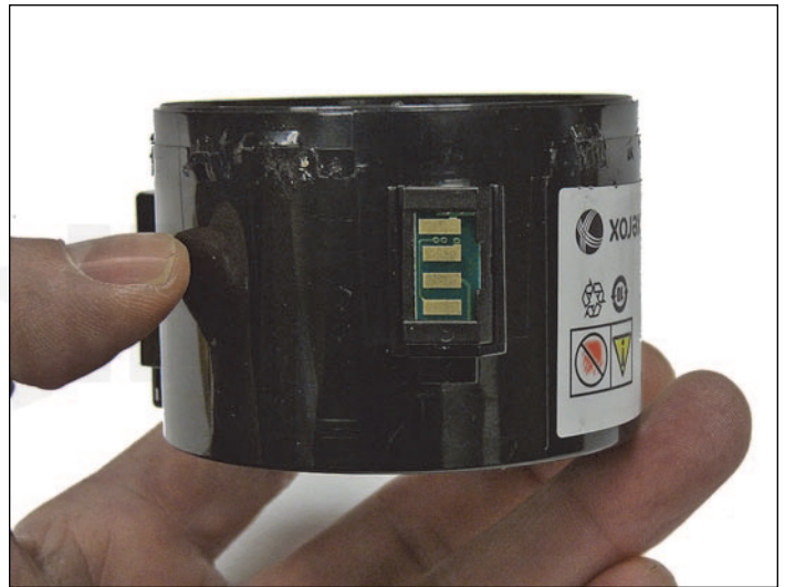
7. Install the chip holder onto the cartridge.
