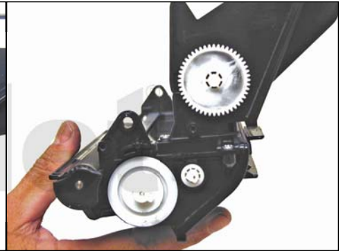
16. On the side opposite the fill plug, remove the two screws and end cap and gears as shown.
