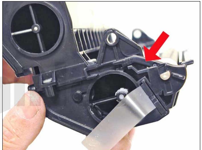
28. Clean the magnetic roller assembly with a dedicated magnetic roller cleaner.
