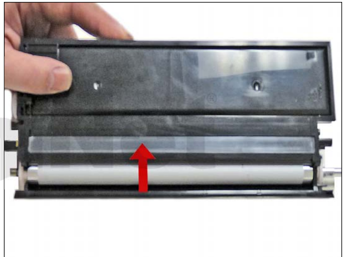
21. Clean the edge of the developer chamber opening with a cotton swab dipped in alcohol. Clean the adhesive off the old seal and replace.
