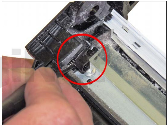
28. Remove the two PCR Holders and PCR-Cleaning Roller Holders, carefully prying them up from the sides.
