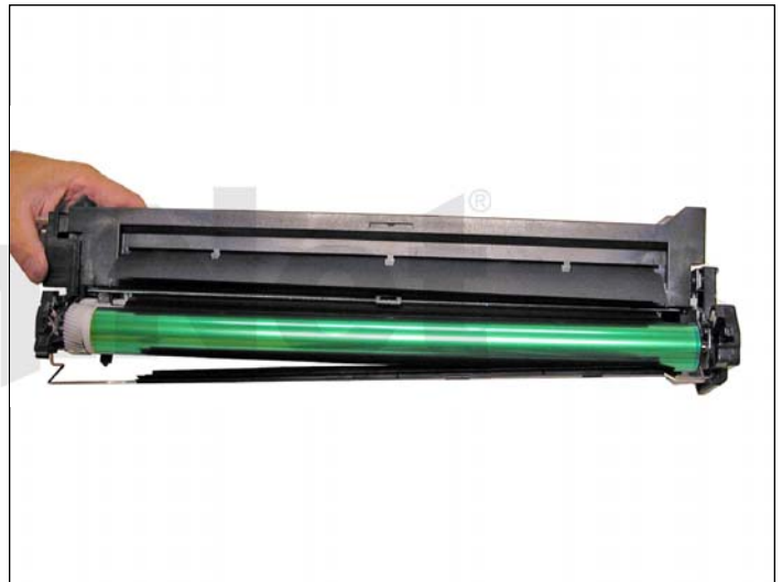
33. Partially install the right end cap/drum/drum cover assembly.
