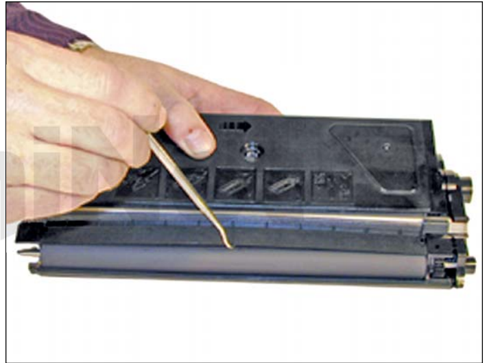
6. Using a spring hook, bend up the middle of the developer roller cover, and remove from the cartridge. The cover has a small plastic tab that locks it in place on each side.
