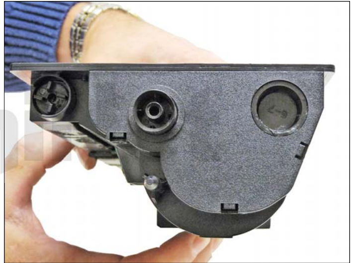
8. Angle the top tabs in first and snap the cover back in place.
