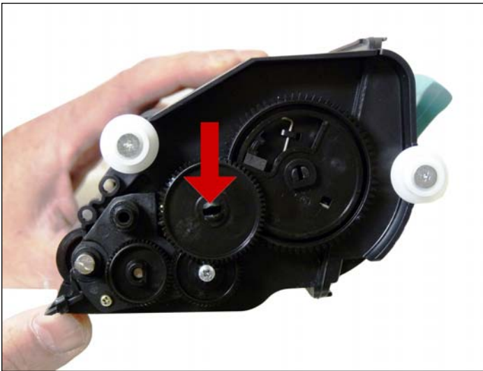
8. Remove the large idler gear by pressing in the two clips in the center of the gear.
