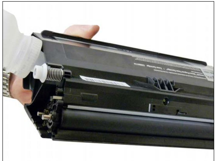
20. Fill the cartridge with the proper amount of E260 toner and install the fill plug.
