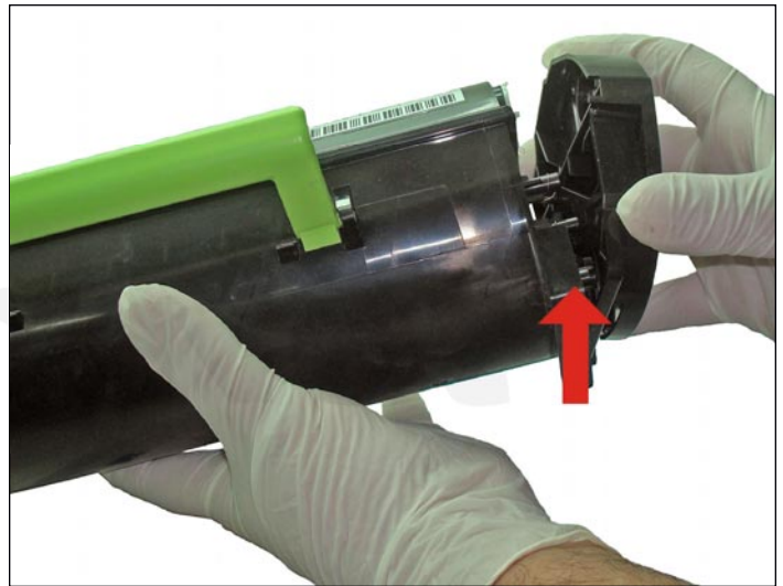
2. Carefully pry open the end cap while holding the push-plate steady to avoid dropping it.
