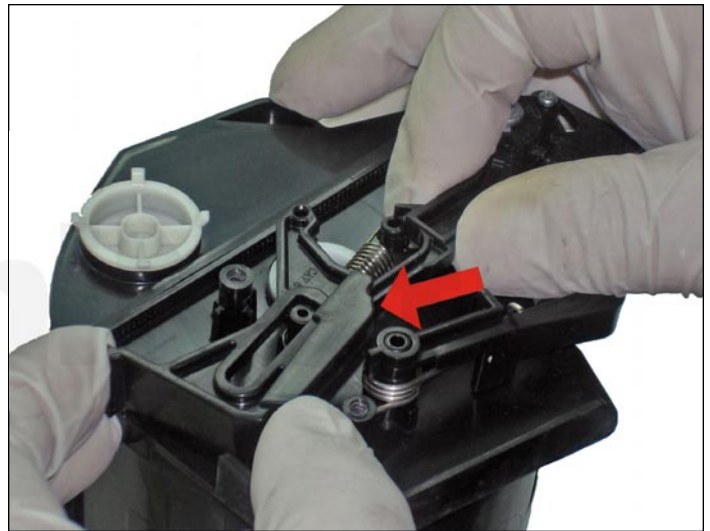
13. Install the push-plate into the sliding guide and insert the tip of the arm inside it.
