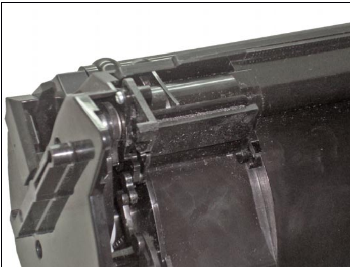
18. Check to make sure the closing and opening of the toner outlet system functions properly. Without pressing the front plate, the toner outlet must remain closed all the time.
