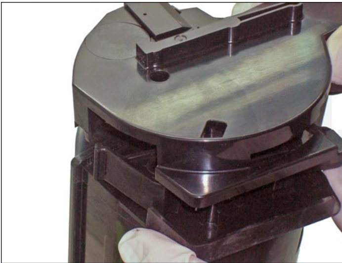
16. While keeping the mechanism pressed against the cartridge to avoid displacement, position the end cap to be seated in its final place.
