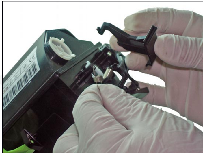
4. Remove the spring at the end of the arm, and lift to remove it from the sliding support.
