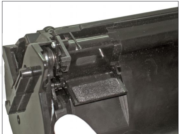
19. By manually pressing the arm (as shown in the photo) or by inserting the cartridge in the machine, the outlet lid must open and close when released.
