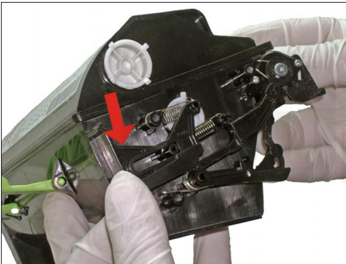
3. Remove the end cap holding your finger on the small plastic arm indicated by the arrow. It is possible that the pushing-rod of the toner-exit lid could come loose, requiring proper seating adjustment during assembly to function properly.
