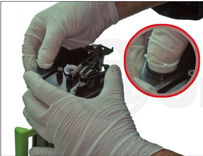
9. Replace the fill plug and check for leaks.
