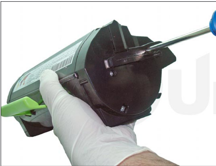
1. Remove the three screws of the right-side end cap of the toner cartridge.
