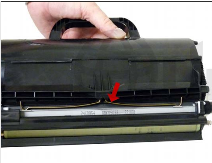
16. Remove the doctor blade spring by pressing down on the center of the spring.
