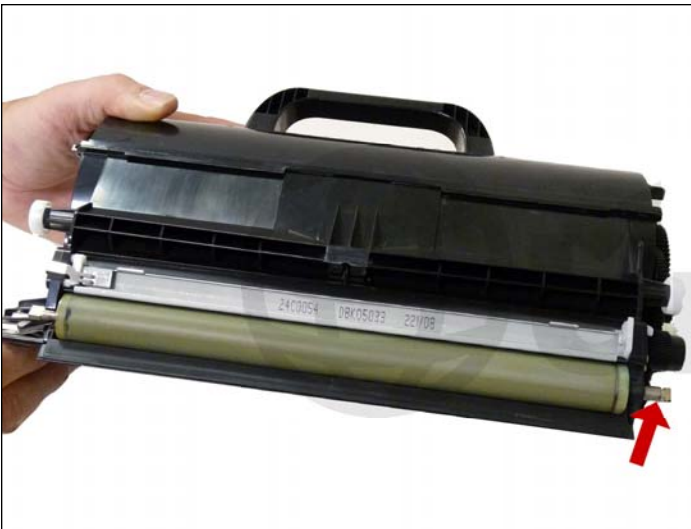
24. Place the longer keyed end of the developer roller into the cartridge and install the roller.
