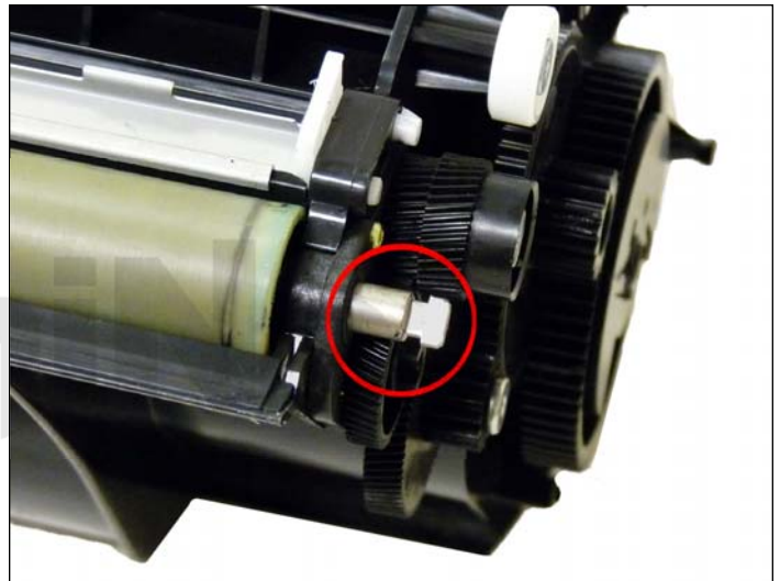
24. Place the longer keyed end of the developer roller into the cartridge and install the roller.
