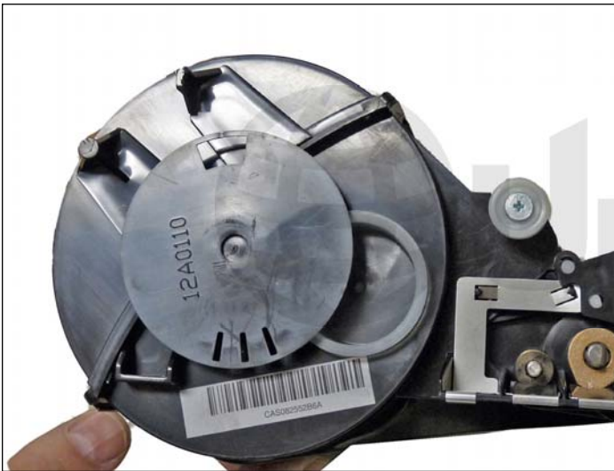
29. Install the encoder wheel.
