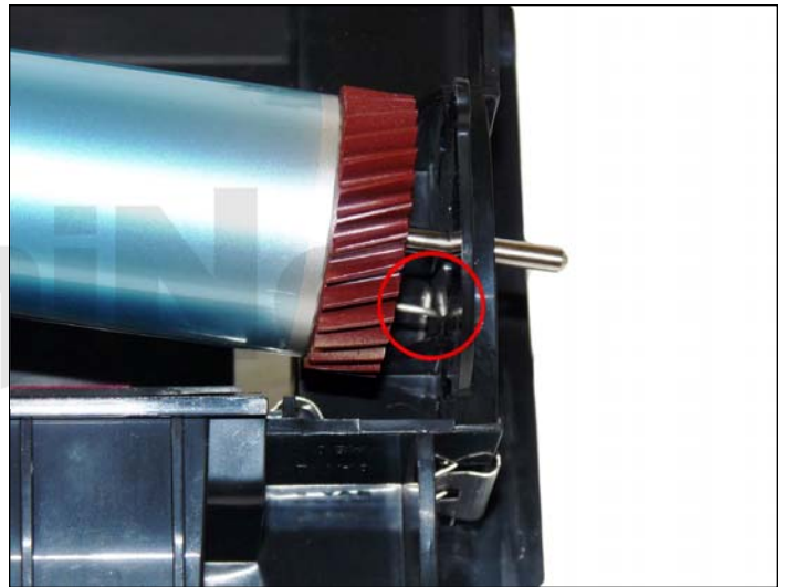
30. Take the OPC drum and lightly coat with your preferred Lexmark drum lubricant. Place the OPC drum into the cartridge with the long thin axle on the contact or non-chip side of the cartridge. Make sure that the spring is in the proper position.
