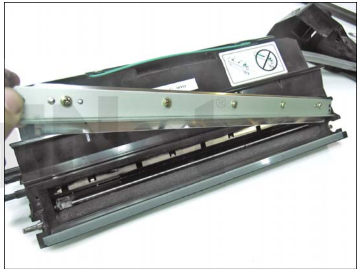
27. Lift the doctor blade out from one side, then to the other.
