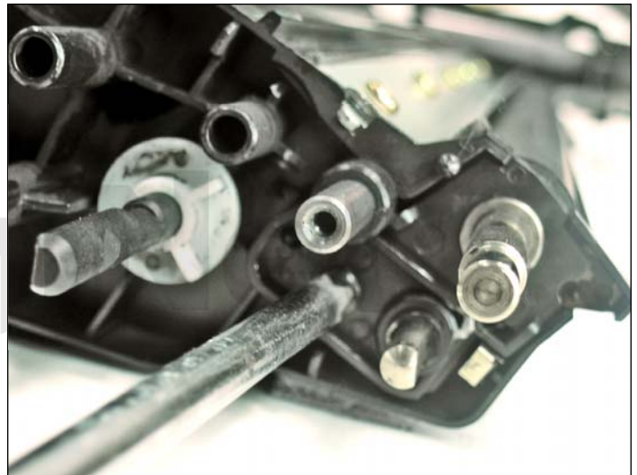
12. Remove the screw to release the gear housing shown.
