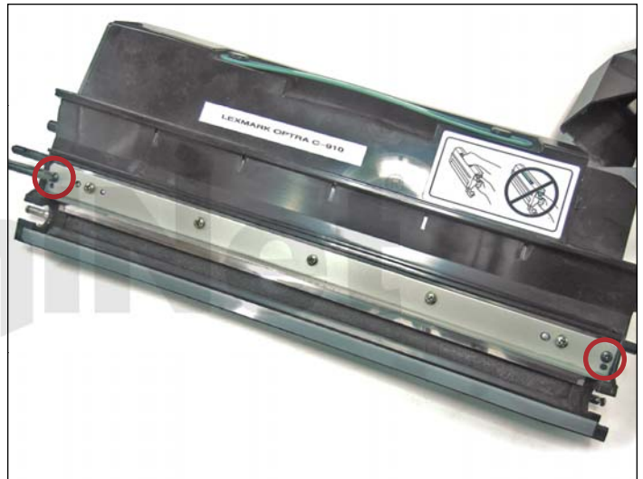
25. Remove the two screws from both sides of the doctor blade shown.
