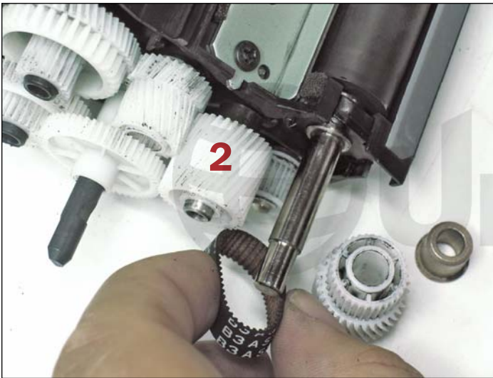
5. Remove the drive belt and gear (#2) shown.
