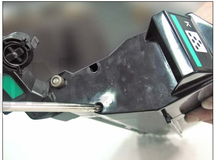
15. Remove the two screws from the end cap on the opposite side of the cartridge.
