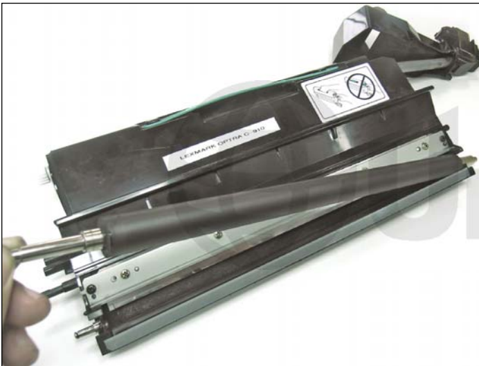
24. Lift the developer roller out from one side to the other.
