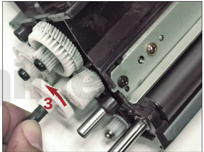
6. Rotate gear (#3) counter-clockwise to unlock and release it
