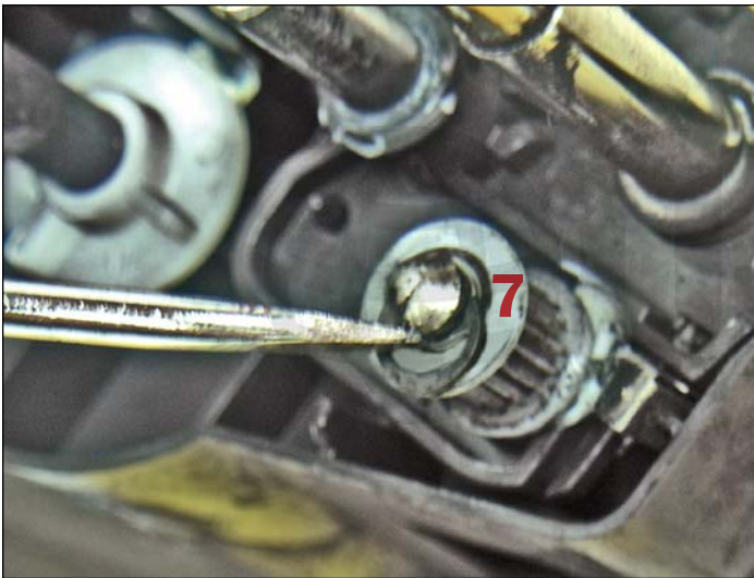
9. First, remove the “C” clip to unlock and release the supply roller gear (#7).
