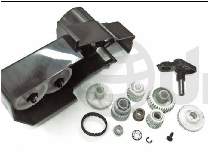
14. Make sure all gearside components are accounted for before proceeding.
