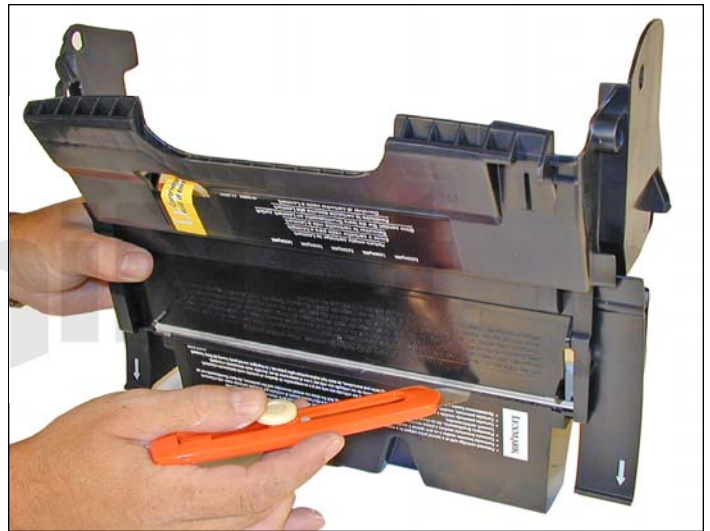
10. The wiper blade is sealed against the waste bin border by way of self adhesive foam in the back edge. This foam should be cut with a razor to release the blade from the cartridge.
