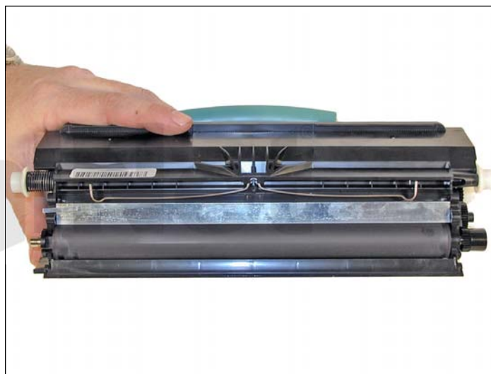
12. Install the doctor blade making sure it is positioned correctly and install the leaf spring.
