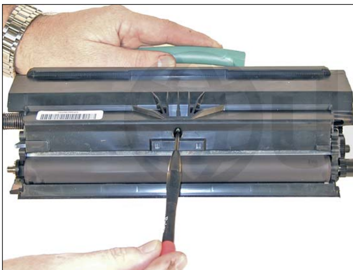
13. Re-install the developer roller cover and screw.
