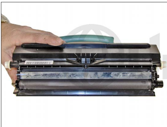
12. Install the doctor blade making sure it is positioned correctly and install the leaf spring.
