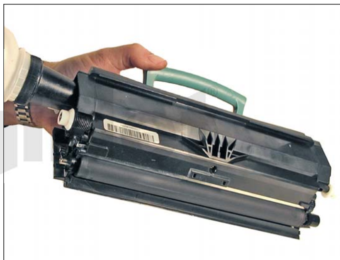
14. Fill the cartridge with the proper amount of toner and install the fill plug.
