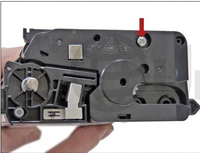
2. Remove the screw from the black end cap on the contact side.
