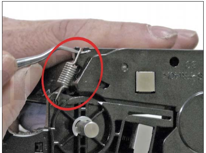
1. Remove the two springs from either side to the cartridge.
