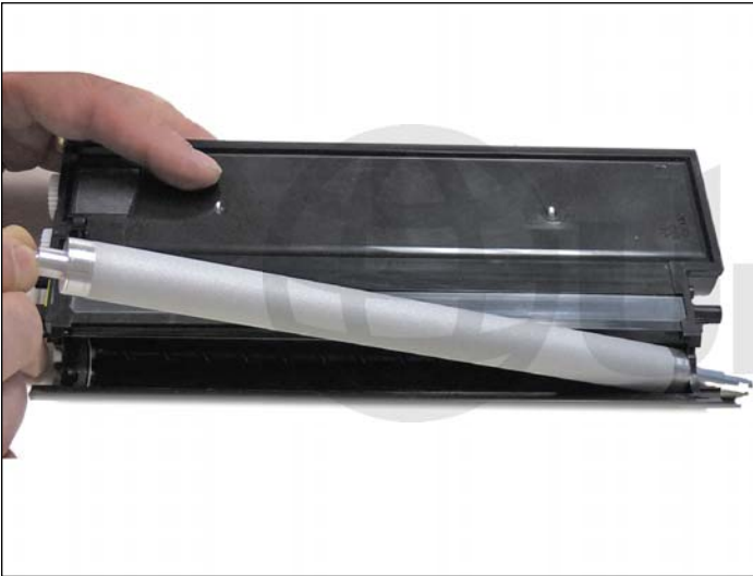
15. Install the magnetic roller long shaft side first.
