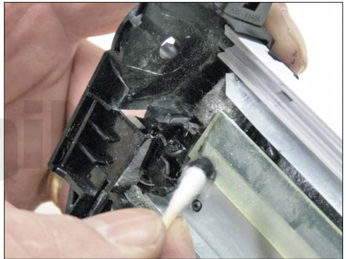
32. Clean the PCR holders and PCR cleaning roller holders with a cotton swab and alcohol.
