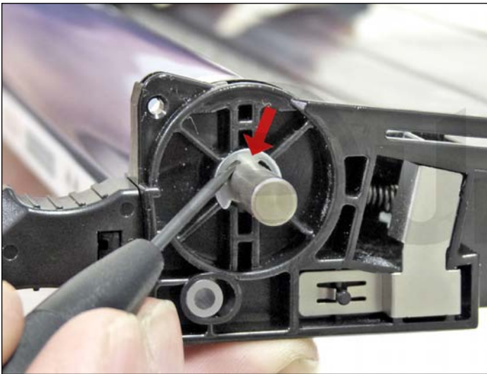
23. On the drum chamber, remove the “E” ring from the contact or hub side of the drum.
