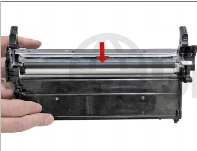
35. Install the cleaned PCR. Place a small amount of new conductive grease on the black holder side.
