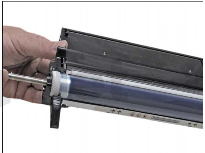
24. Pull the axle out from the gear side of the drum so that the inner drum ground contacts are not damaged.
