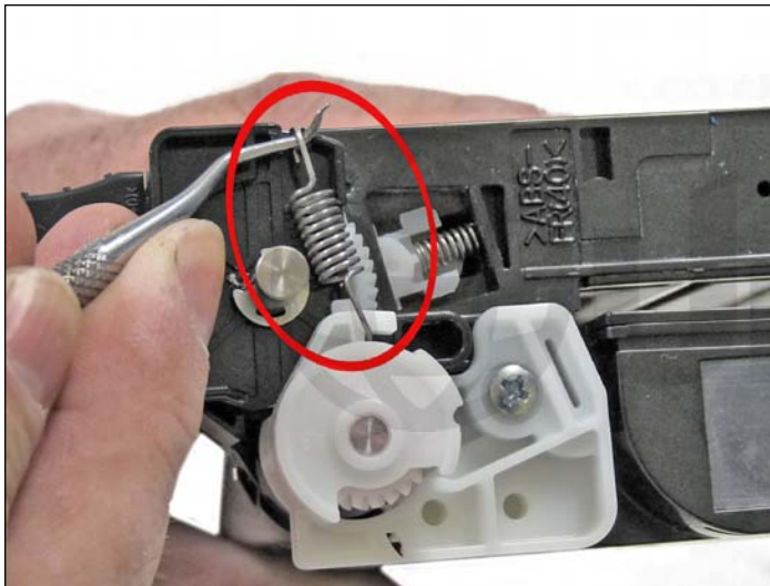
1. Remove the two springs from either side to the cartridge.
