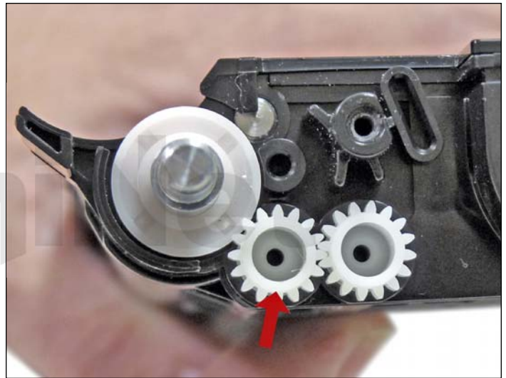
18. Install the front auger gear. Make sure it is installed correctly. It must mesh properly with the auger or print voids will occur.
