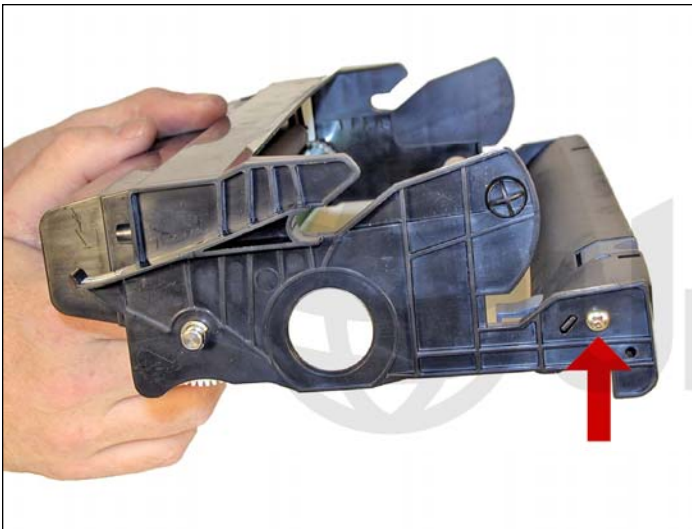
14. Install the handle/cartridge lock assembly and two screws. Just to make sure that everything is meshing properly and lubricated properly, rotate the drum by the large gear in the proper direction. This is always a good idea for drum units as a final check before installing the cartridge in your test machine.
