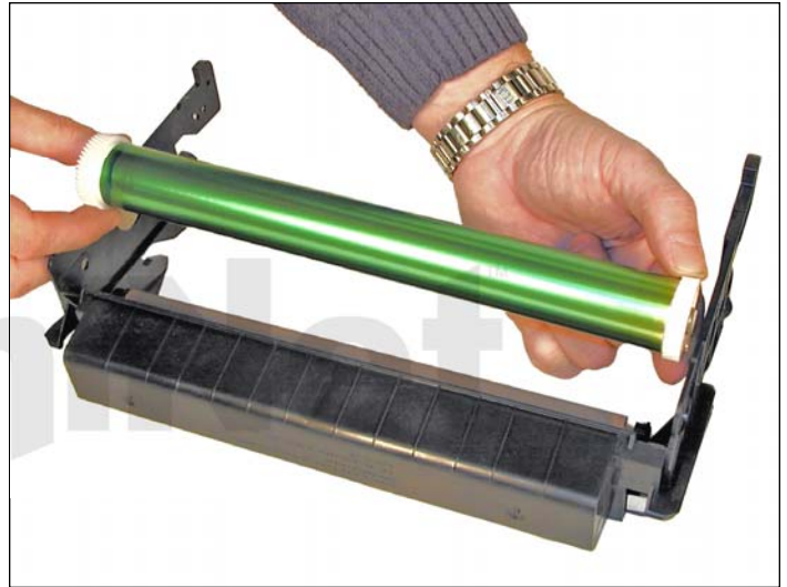
11. With the waste chamber facing you, install the drum so that the large gear is on the left side, spring on the small gear facing down.
