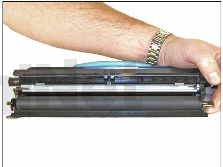
11. Wipe the developer roller with a clean lint free cloth, and re-install the developer roller. At this point we do not recommend that any chemicals be used to clean this roller.
